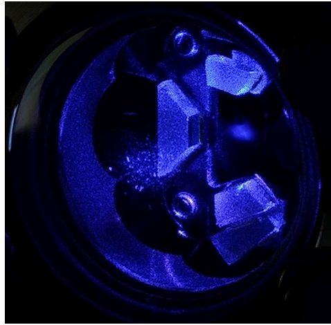
Figure 23.9: Picture of a strontium MOT operated at 461 nm. The atomic cloud, which consists of about 10^6 atoms at 5 mK temperature is visible as a diffuse spot located inside a three-mirror ring cavity.
