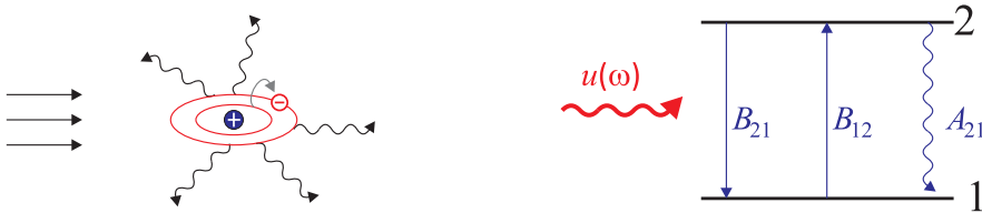
Figure 1.10: Bohr model and Einstein rate diagram.
