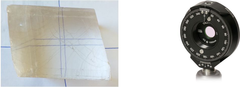
Figure 27.10: (Left) Transmission through a birefringent crystal. (Right) \lambda/2 -waveplate mounted in a rotation stage.
