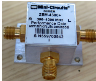
Figure 28.16: Picture of a radiofrequency mixer.
